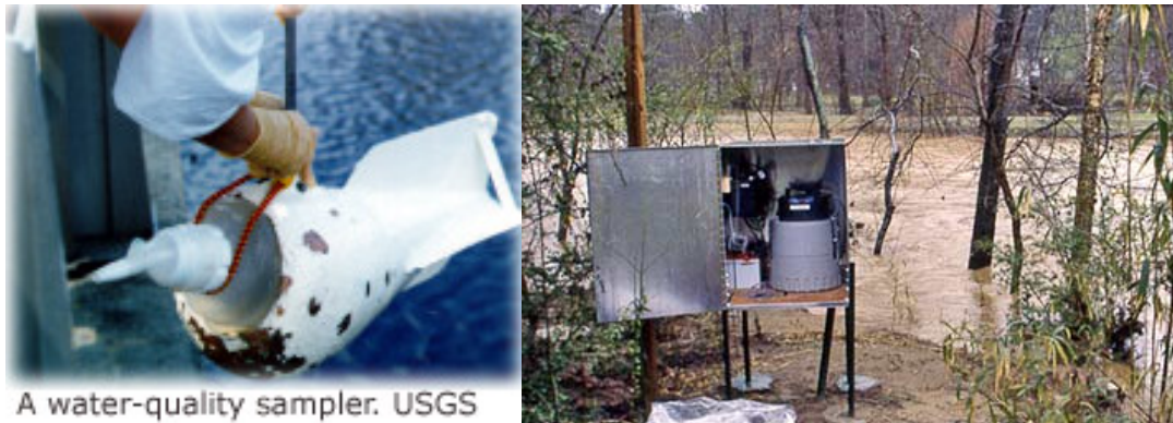
Figure 1 – Left: Depth integrating water quality sampler ( http://ga.water.usgs.gov/edu/qwsampler.html ), Right: Autosampler that can be set to sample at fixed time intervals, or flow levels ( http://ga.water.usgs.gov/edu/autosampler.html )
